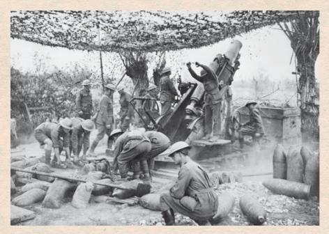
A 9.2inch howitzer of 55th Australian Siege Battery in action at Voormezeele, 13 September 1917. The four men to the rear of the gun lift the shells to the piece in a metal frame. An overhead net provides concealment from the air. (IWM E.AUS.964)
