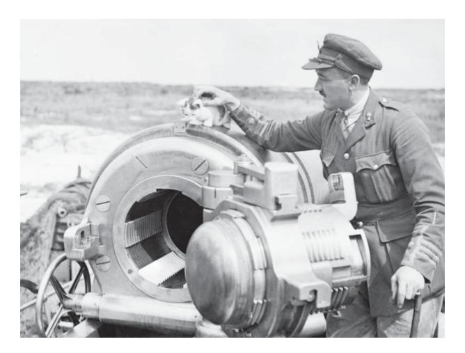
A gunner major at the awesome breech of a 12-inch howitzer of 444 Battery, Royal Garrison Artillery, near Arras, 19 July 1918. The weapon weighed well over 20,000lb, and 20 tons of soil were loaded into its 'earth box' to counteract the massive recoil. The officer's rank is denoted by the crown and three lines of lace on his cuff: a gold 'wound stripe' worn above his rank insignia shows that he has been wounded once. (IWM Q6873)
