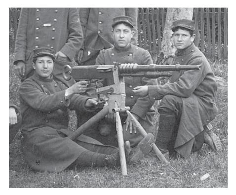
French gunners with the 8mm Hotchkiss machine gun. The air-cooled Hotchkiss was a reliable weapon, usually fed from strips of 24 or 30 cartridges. Despite the lack of a water jacket the equipment was still heavy – with the gun and the mount weighing about 53lb each. (Author's collection)
