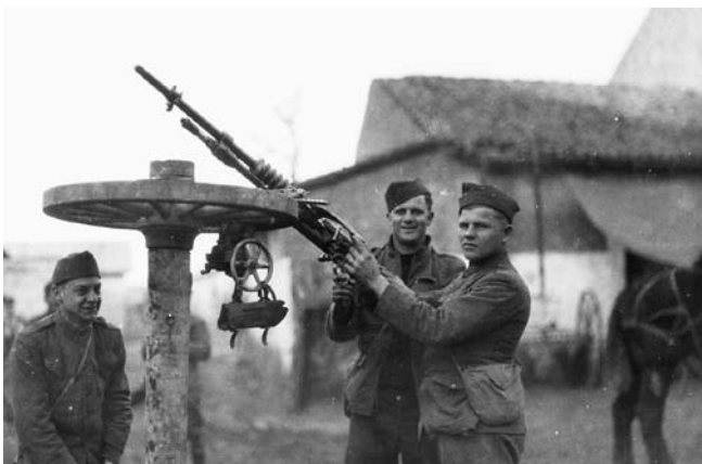
6-18 An old wagon wheel made into a solid revolving base for the Hotchkiss antiaircraft gun.
