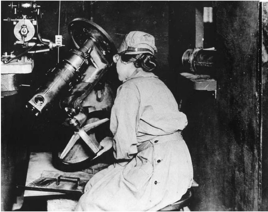
8-25 A woman welding a cylinder of a Liberty ship engine at the Nordyke and Marmon Company, a plant in Indianapolis, Indiana.
