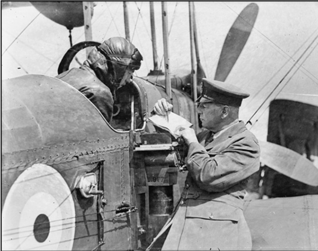
Figure 11: A Royal Air Force officer showing a reconnaissance pilot the area to photograph. The aerial camera is attached to the plane, underneath the map. (Chapter 8 )
