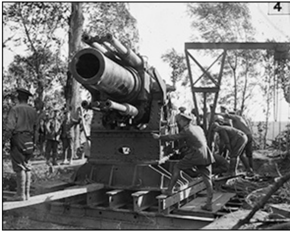
Figure 6-2: A British 15-inch howitzer ready for action on the first day of the Battle of the Somme. Howitzers fired shells high, so they were ideal for bombarding enemy positions.
