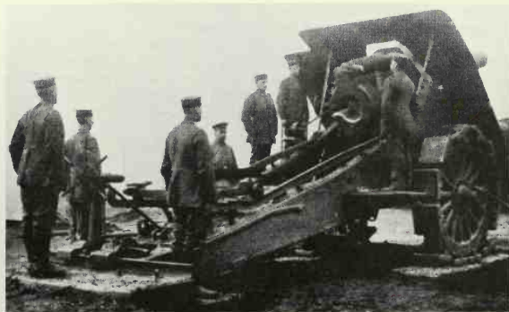
German coast artillerymen in position with a 14-caliber, 280mm Krupp howitzer adapted from a short naval gun, with wheeled mount and wheel belts. It weighed 33,571 pounds complete and fired a 628.4-pound shell more than 10,000 yards.
