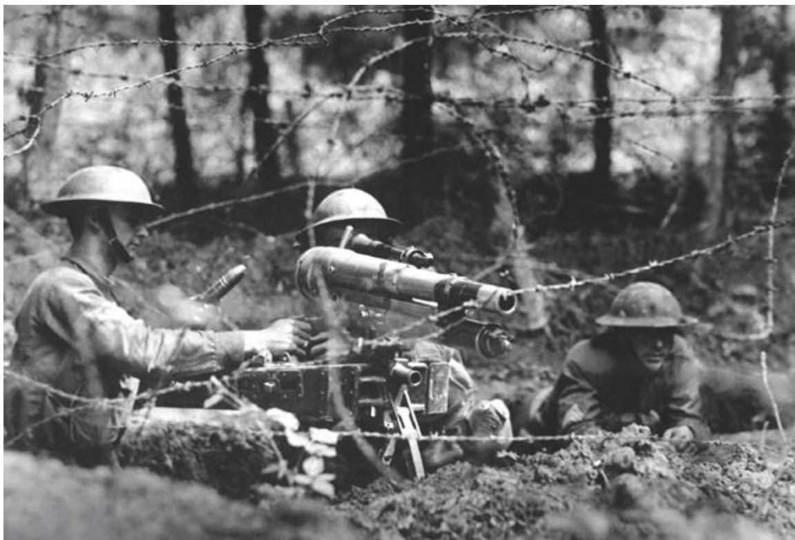
American troops operating a French "37" in a firing position on a parapet in a second-line trench. The gun had a maximum range of a mile and a half, was more accurate than a rifle, and was capable of firing 28 rounds per minute.
