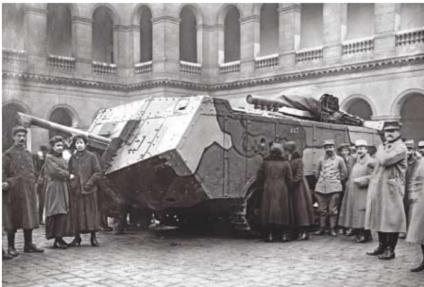
A French Saint-Chamond tank. Its main armament was a 75-mm gun, with four Hotchkiss machine guns as secondary weapons.
