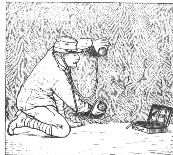
The French listening device improvised from a water bottle. From École de Mines, Supplément au Livre de l'Officier , 1917.
