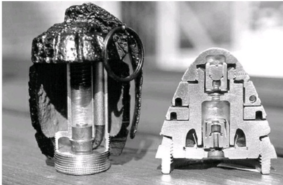
Fig. 7.4: Battlefield souvenirs for sale on the Somme. Grenade and fuze-cap sectioned to show internal mechanism.
