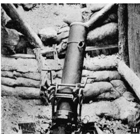
Loading sequence: 1, the catch of the 9.45-inch trench mortar is released enabling it to be revolved 2, 3, 4, 5. The barrel is lowered and the weapon is loaded 6; it is then raised 7 and swung back to its former position 8, 9, 10. The crew retire 11 and the weapon is fired 12. 213GP 214GP
