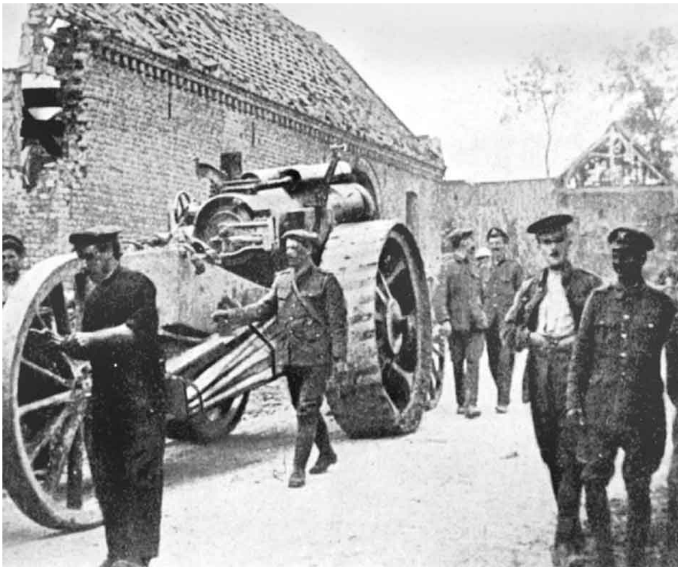
When 8-inch howitzers required moving the American-built Holt agricultural tractor with petrol engine and crawler tracks did the job. 44BP
