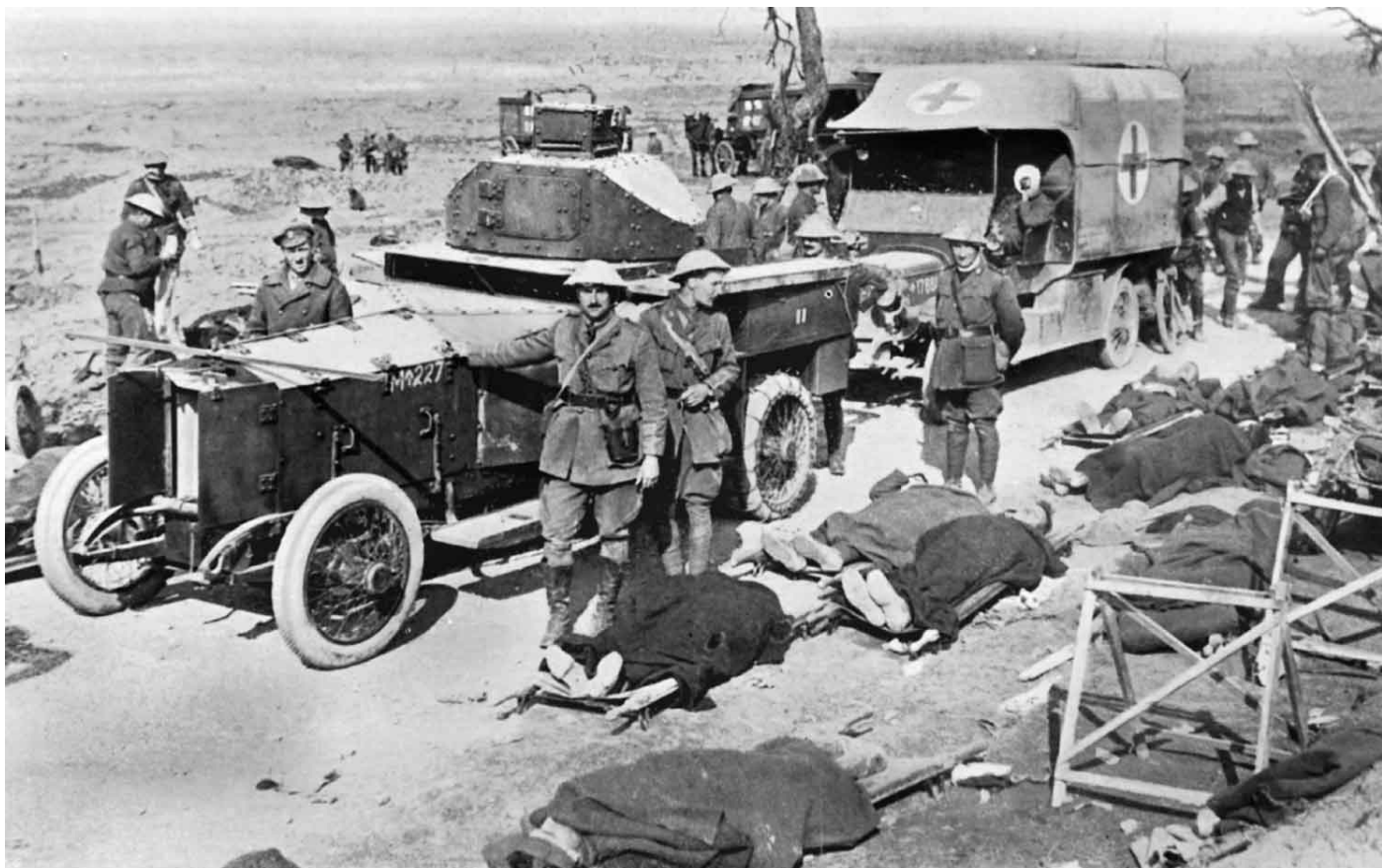
A scene near Guillemont, a Rolls-Royce armoured car among the ambulances. Note the chains on the rear wheels to give traction through mud. 33BP
