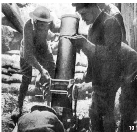
Loading sequence: 1, the catch of the 9.45-inch trench mortar is released enabling it to be revolved 2, 3, 4, 5. The barrel is lowered and the weapon is loaded 6; it is then raised 7 and swung back to its former position 8, 9, 10. The crew retire 11 and the weapon is fired 12. 213GP 214GP
