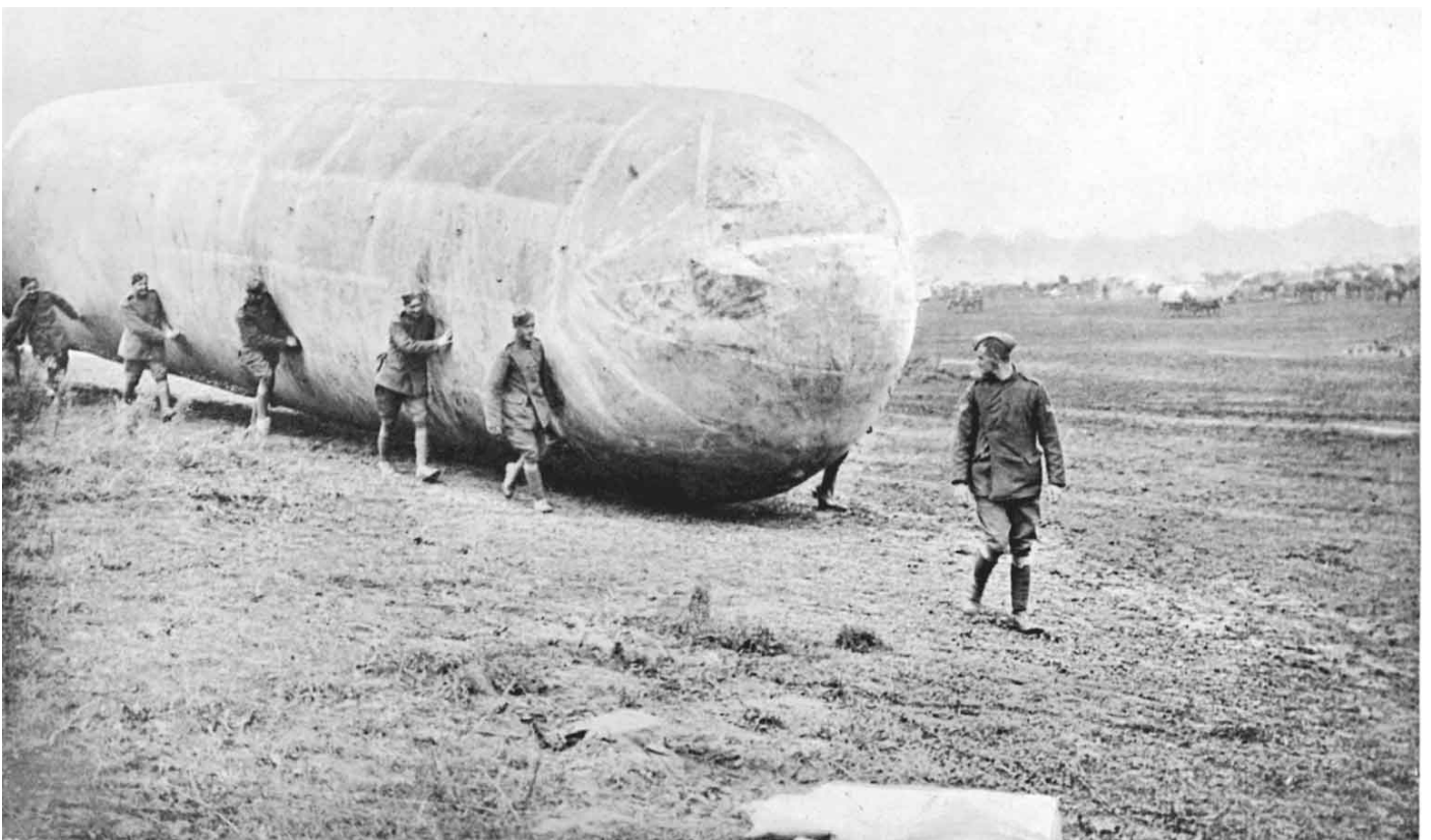
Men of the Royal Flying Corps bringing up a 'nurse balloon'. It was used to transport the large quantity of gas required to inflate an observation balloon. 55BP
