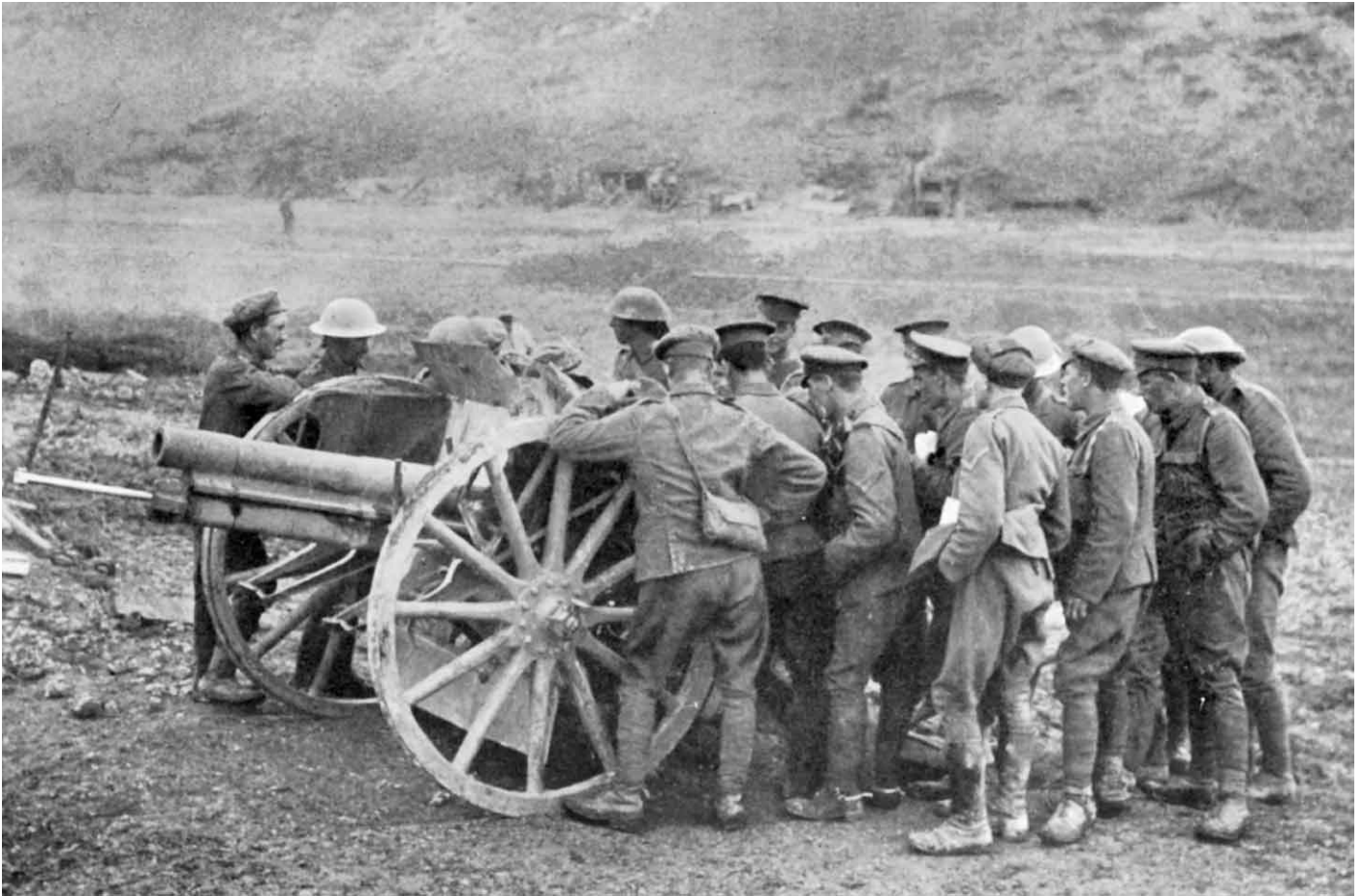
Artillery men examine a captured German 77mm Field Gun M96nA. This was the principal field gun built by Krupp and was used throughout the war. 116BP
