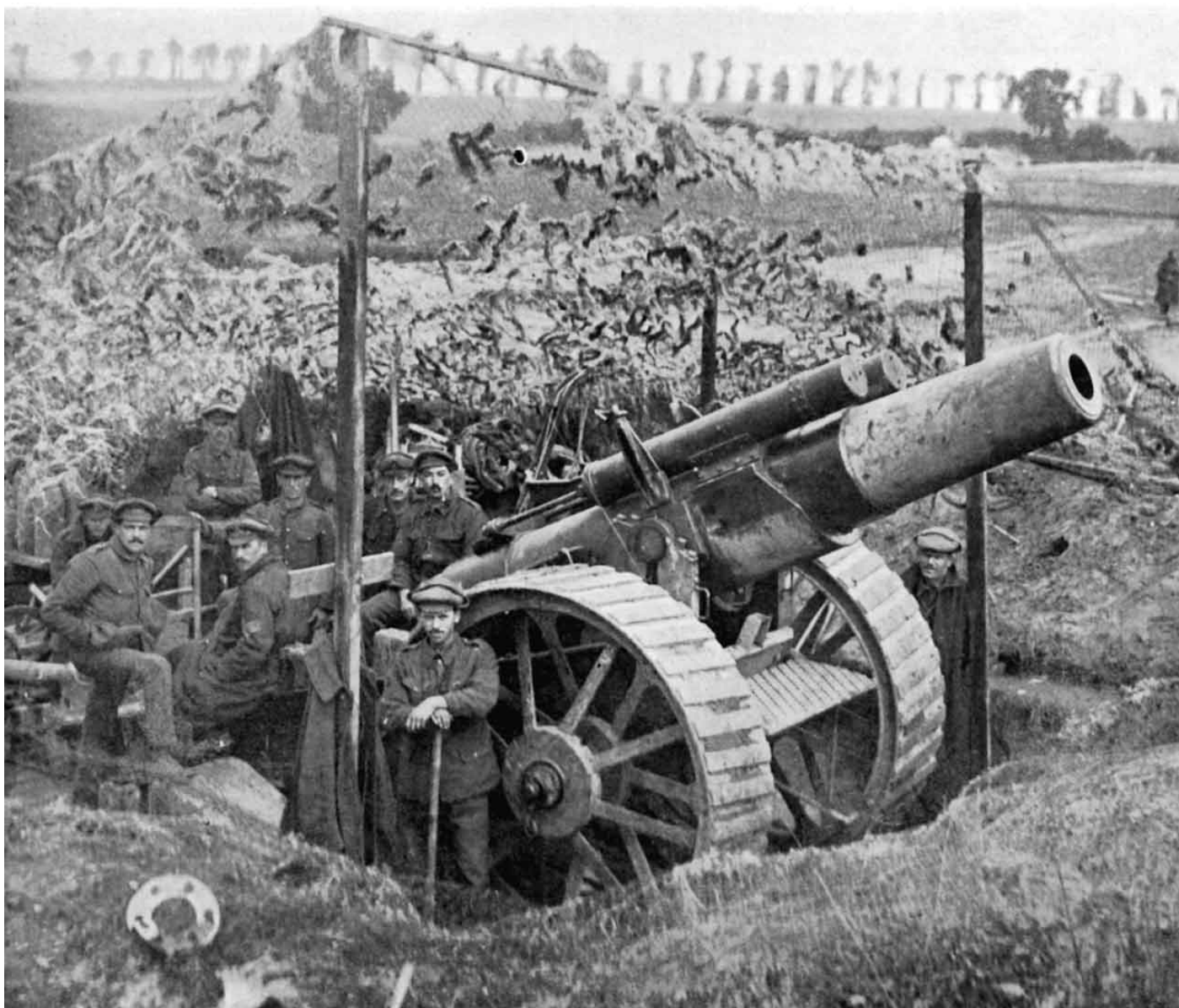
The BL 8-inch howitzer Mark I, a British improvisation developed to provide heavy artillery. It used shortened and bored-out barrels from various redundant naval 6-inch guns. It remained in use on the Western Front throughout the war. 121BP
