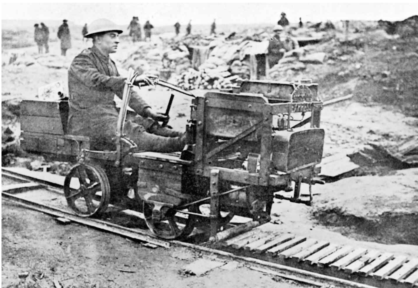
The Scotch Express was one of the earliest petrol tractors used over the light railway system and it was made from motor car parts. 336GP
