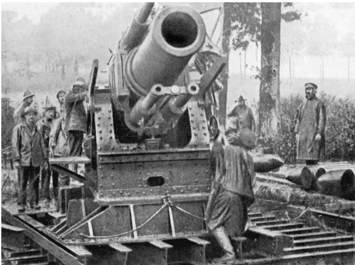
Ramming home a shell into the breech of the 12-inch Mk1 howitzer, or 'Grandmother', manned by the Royal Marine Artillery. 203GP
